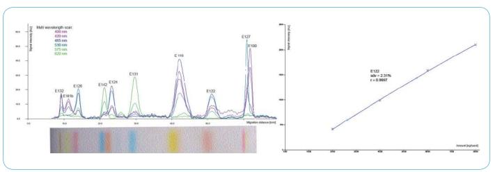
Fig. 3: Multi wavelength scan of a food additive mixture (absorption curve overlay of 6 wavelengths); exemplarily shown is the calibration function of E122 (x) found in a fruit drink sample (+)
