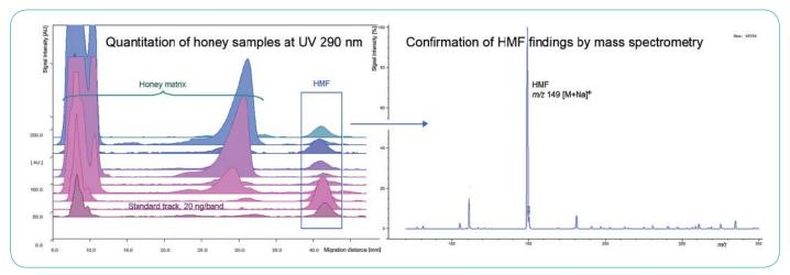
Fig. 2: Fast and reliable HPTLC analysis of hydroxymethylfurfural (HMF) in honey samples
